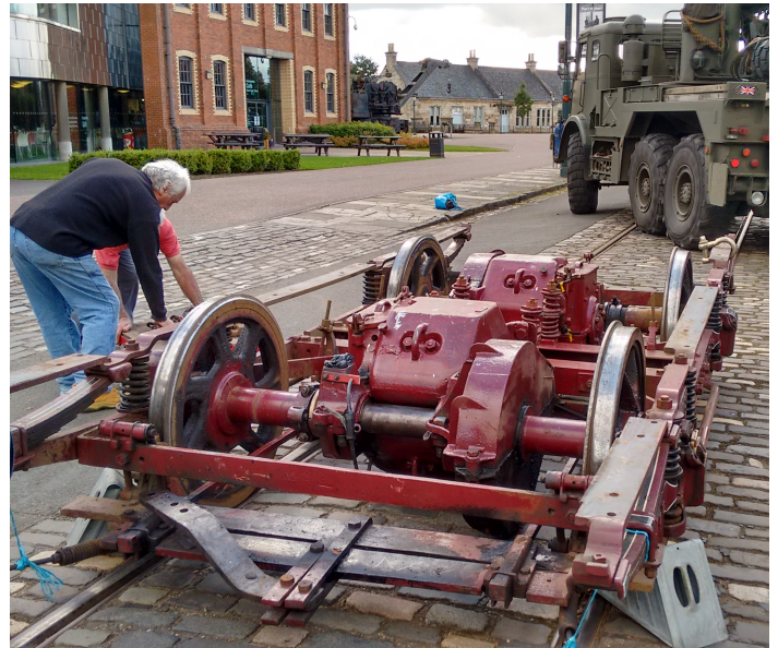
Charlie prepares 1017s bogie for lifting off the tracks
