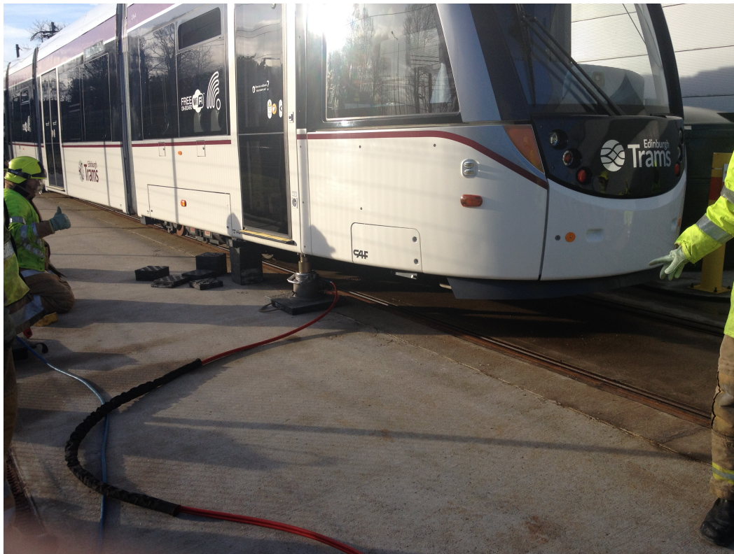
Edinburgh tram is jacked up
